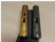
Note the spur gear recess is different between the MAX and Super Max as well as the Super Max having the full length cylinder.
