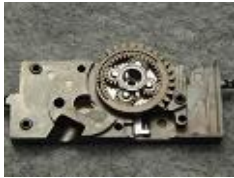
Satellite gear system inside the sector gear. Note: this is from the Max version where there is only one single stainless steel gear. The Super Max version offers all 4 stainless steel gears.
