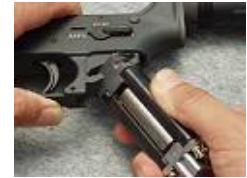
Due to the way the motor is secured on to the PTW, this is extremely sturdy and will not require re-alignment like most AEGs.
