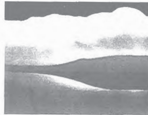
Figure 7.8 SEM micrograph showing the cross-section of the bird's beak due to oxide encroachment (Ref. 9, © 1981 IEEE).
