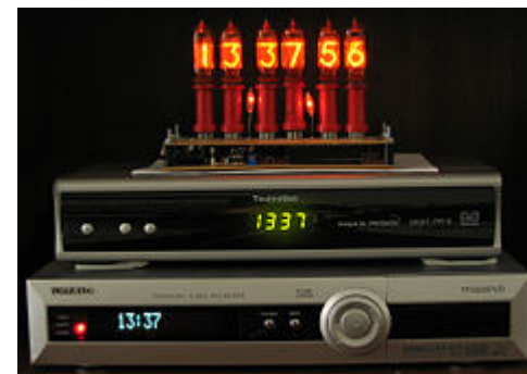
Nixie tubes, LED display and VF display, top to bottom
