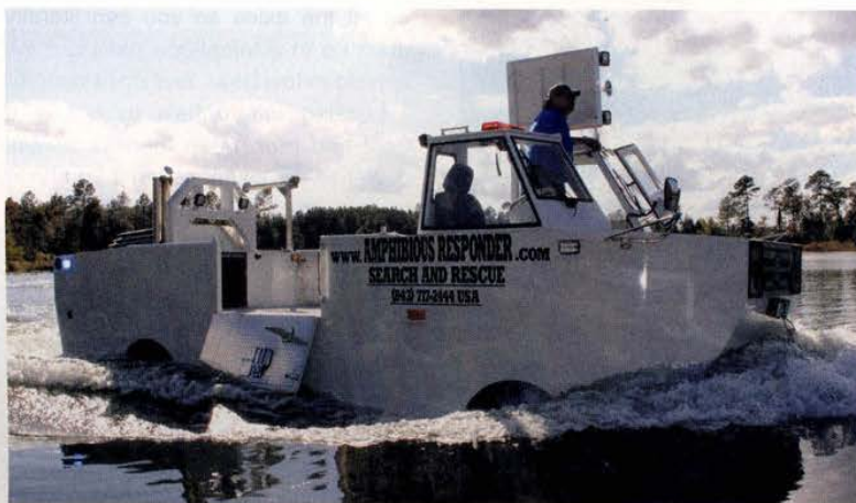
CAMI delivered its first amphibious responder to the city of Bangkok, Thailand. That model incorporates Ford's 6.7 L Power Stroke diesel engine and a 6.7 L Cummins MerCruiser QSB6.7 diesel marine engine.
