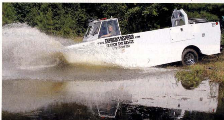
The hull of the amphibious responder is constructed of high-tensile, marine-grade aluminum alloys and is designed to absorb and deflect energy from rough impacts.
