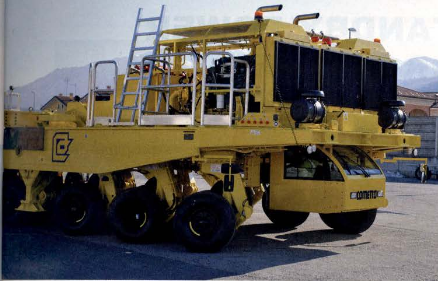
One of two Volvo Penta TAD765VE engines can be seen in the Cometto AIT250 hauler.
