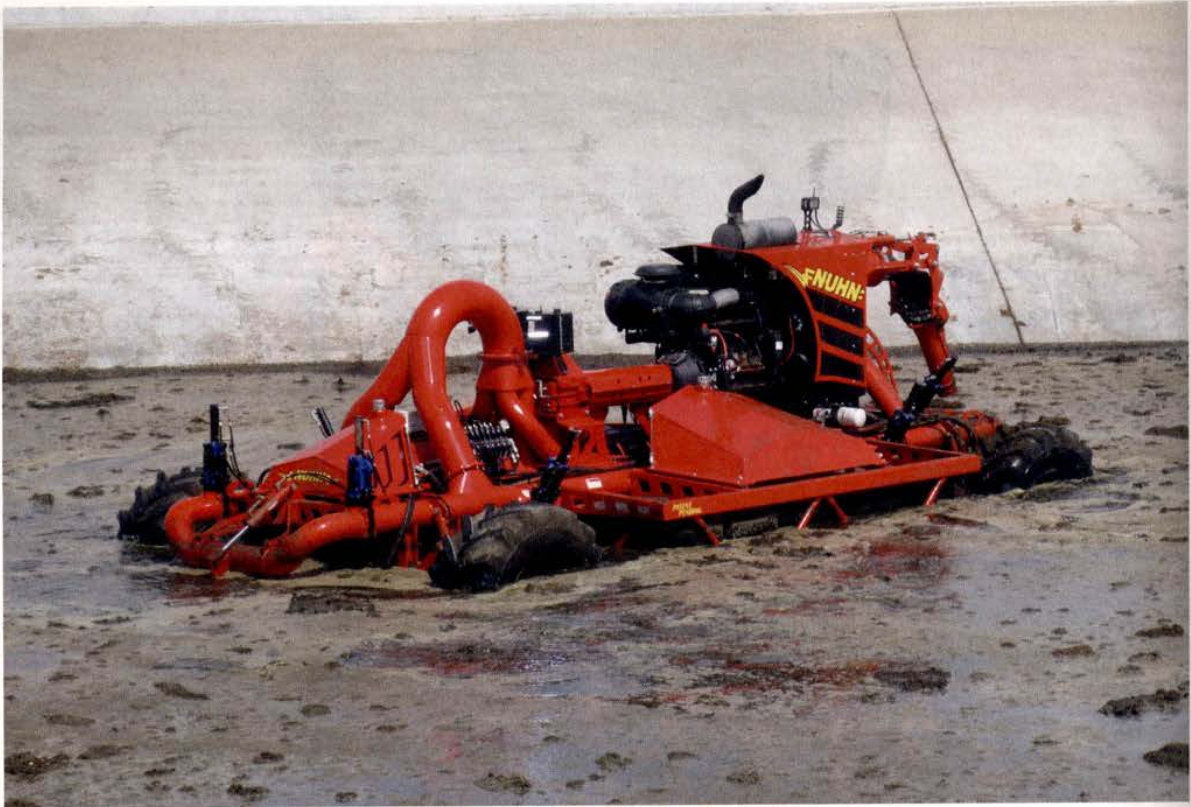
A 270 hp Cummins QSB6.7 diesel engine sits high above the surface of the manure pond. It drives a hydraulic system on land as well as pumps and agitators for propulsion and directional changes while at sea.
