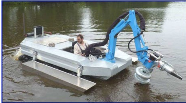
6-Wheel driven unit with stabilizer pontoons
