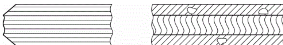
Figure 12 — Arrissed edge (with blank spots)
