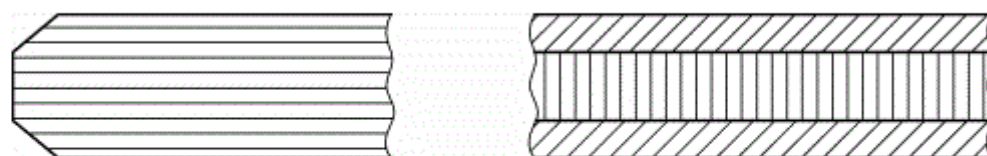
Figure 14 — Smooth ground edge (no blank spots)
