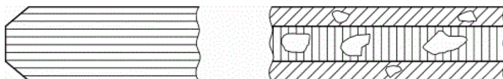
Figure 13 — Ground edge (with blank spots)
