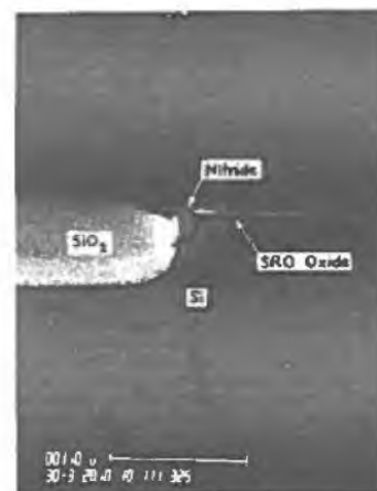
Figure 7.14 SEM micrograph showing the cross-section of a SWAMI structure (Ref. 10, © 1982 IEEE).
