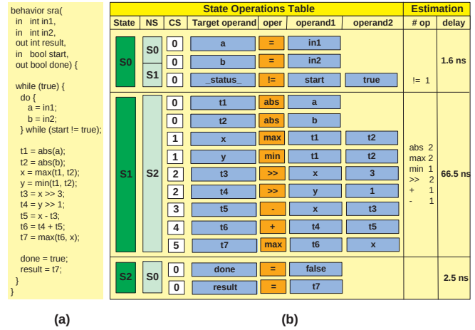
Figure 7. Square root approximation example (a) behavioral C/C++ code (b) SFSMD
