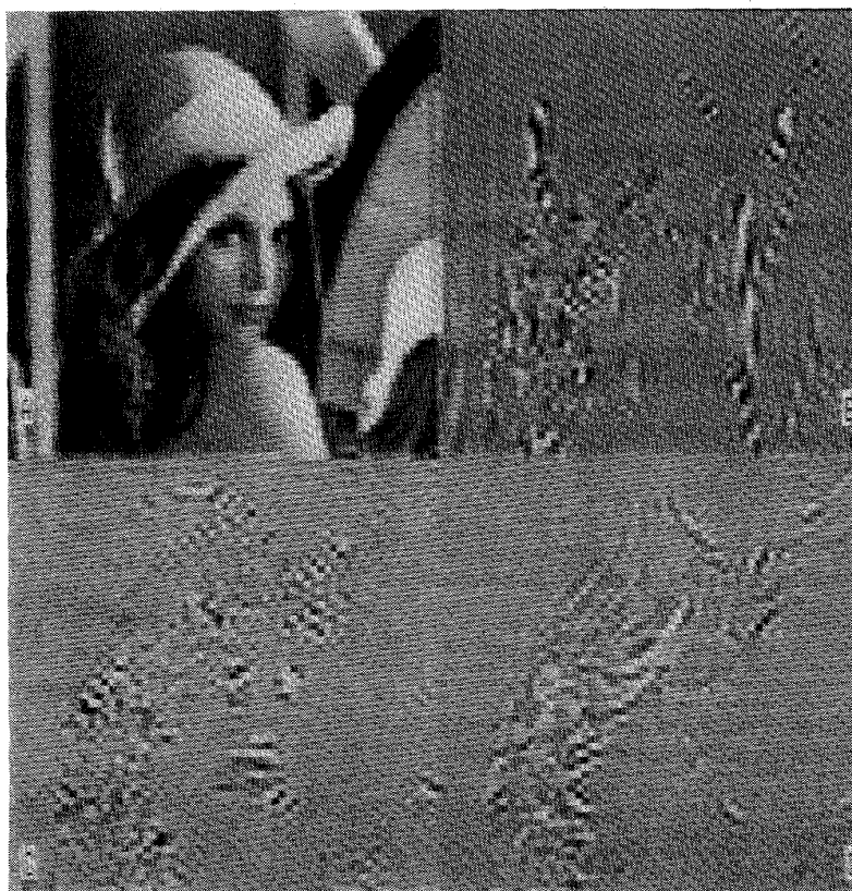
Fig. 6. Some subband signals of "Lady" image: (a) subband 11-11, (b) subband 11-21, (c) subband 11-12, (d) subband 11-22 (zoomed by 2 \times 2 ).
