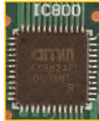
AMS AS3824E (16-channel LED TV backlight controller)
