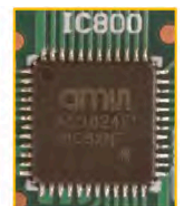
AMS AS3824E (16- channel LED TV backlight controller)
