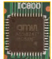
AMS AS3824E (16- channel LED TV backlight controller)
