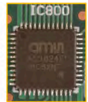
AMS AS3824E (16- channel LED TV backlight controller)
