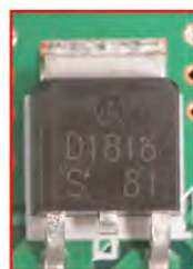
ON Semi D1816 NPN Bipolar transistor
