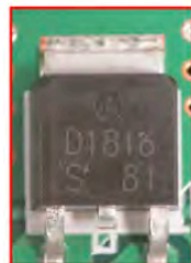
ON Semi D1816 NPN Bipolar transistor
