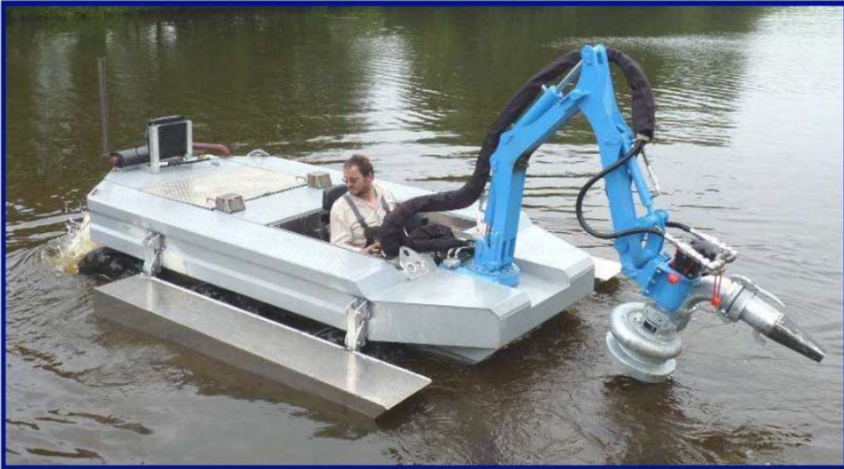
6-Wheel driven unit with stabilizer pontoons
