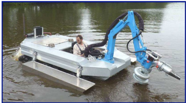
6-Wheel driven unit with stabilizer pontoons
