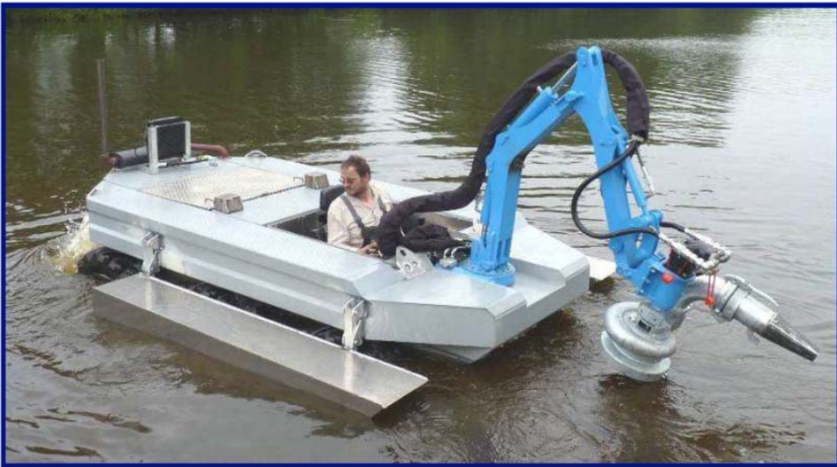
6-Wheel driven unit with stabilizer pontoons
