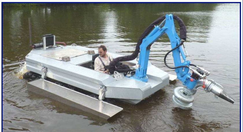
6-Wheel driven unit with stabilizer pontoons
