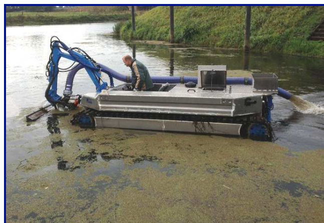
Suction an pumping of swimming algae and weeds
