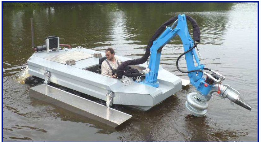
6-Wheel driven unit with stabilizer pontoons
