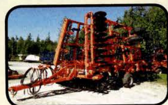
KRAUSE 6440 24' LANDSAVER, 9" EDGE ON SPRING SHANKS, 10" SWEEPS, 3 ROWS TINE HARROWS, ROUND REEL, HYDRAULIC GANG ADJUSTMENT, $62,300
