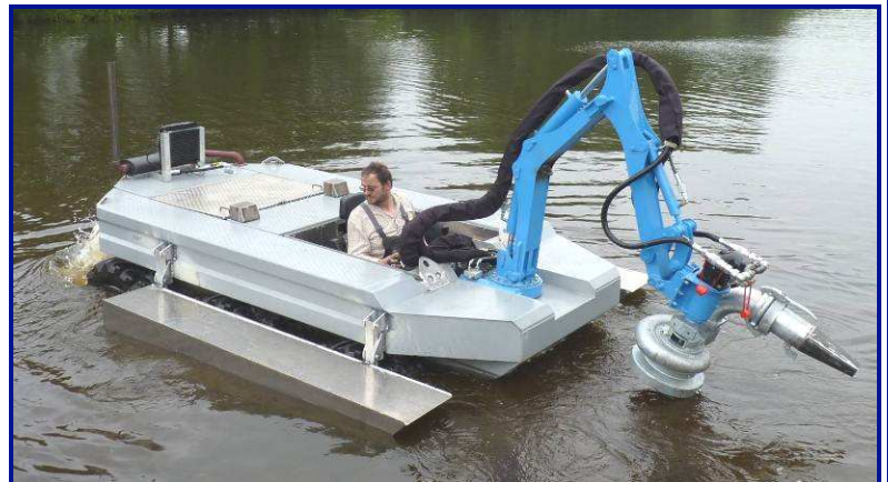
6-Wheel driven unit with stabilizer pontoons
