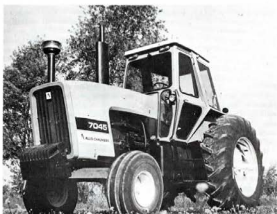
New 145 PTO hp 7045 is available with new Acousta cab II and 20 speed Power Director transmission with 2-speed shift-on-the-go capability. It's powered by a 145 hp diesel. The new 7020 has a 120 hp engine.
