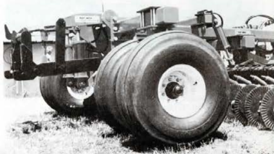
Ruff-Neck "Load Lugger" features 3-pt. hitch and auxiliary toolbar on which coulters or other attachments can be mounted to combine several operations into one. Chemical tank for pesticides or fertilizer can be mounted on top the unit.
