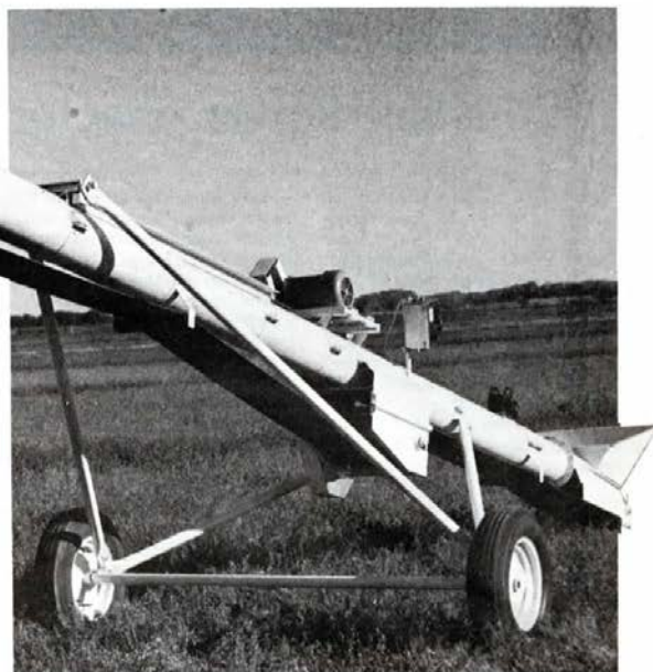
Belt conveyors (12 in. belt) available in standard lengths from 20 to 60 ft.
