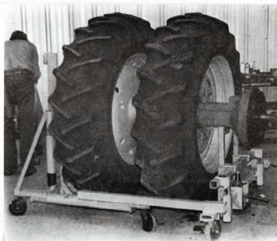
Dual tire adapter fits on Cofer's single tire cart, allowing one man to remove a set of duals with the final drive housing attached. Rated at 8,000 lbs. capacity.
