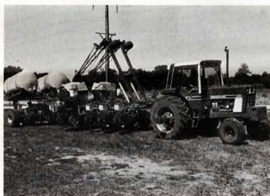
The tractor moves forward and the tongue elongates to fold the planter wings forward for transport. Frame, available in 30 to 60 ft. widths, accommodates new or used planter units, wheels, drives, lift mechanism, frame and marker from 500 Cylco or Deere 7000 or 7100 planters. Said to turn shorter than any other planter toolbar on the market and flexes in three sections. Note how planter is pulled from 3-pt. hitch in both field and road position. There are no hydraulic lines to disconnect in folding or unfolding the unit.
