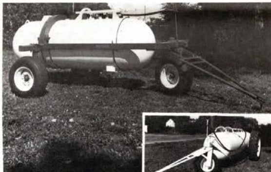
The Torpedo (lower right) has a 10,000 lb. test axle built right through the tank. The Row Rambler handles a 500 or 1,000 gal. tank.
