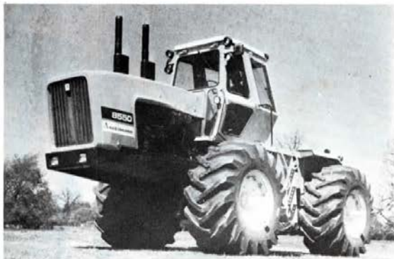
A 300 hp engine powers the new 8550, biggest in the Allis Chalmers line.
