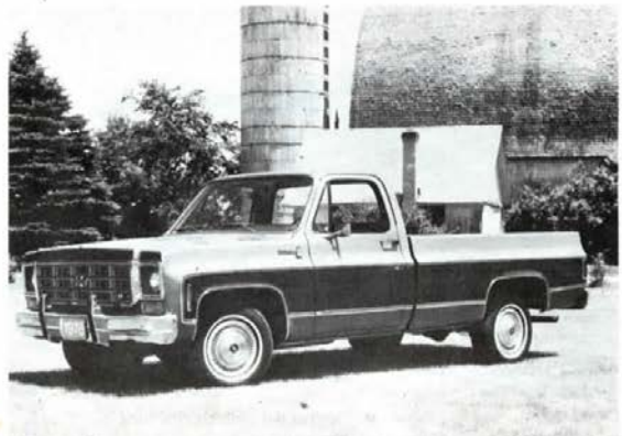
Chevrolet is offering, for the first time in '78, the new GM V8 diesel engine in the half-ton (C10) two-wheel drive Fleetside and Stepside pickups. It develops 120 hp at 3600 rpm and has a compression ratio of 22 to 1.
