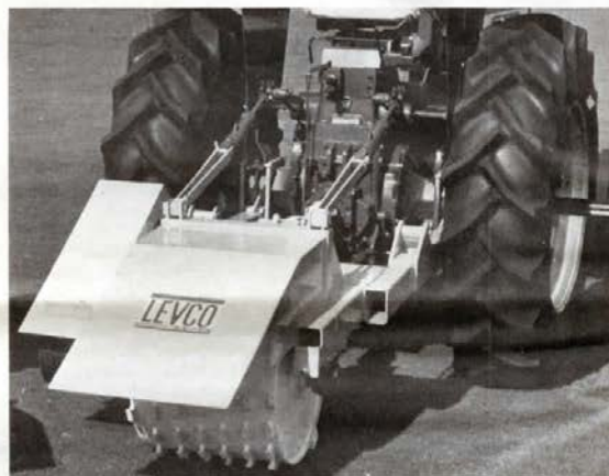
Equip your tractor with the model TW 1000 and you're "tooled up" and ready to do your own and custom stump grinding. Takes a 25 in. wide cut.
