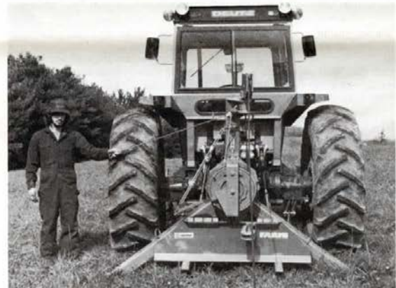
Pulling capacity of the Farmi winch is usually sufficient to pull out a stuck tractor or combine with straight line pull. Heavier objects can be moved with an auxiliary pulley shown in drawings.
