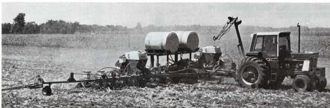
Photo shows Shoup planter frame equipped with 16 Cylco planter units spaced 36 in. apart. It flexes in three sections and has 5 planter units on the outer sections, and 6 on the center section.
