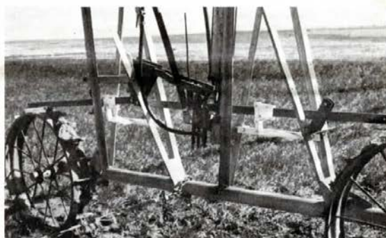
Lug Hopper attachment reduces wear at the high-wearing point of the lugs by eliminating the dragging of the trojan bar dogs over the wheel lugs.
