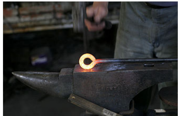
Blacksmiths work iron when it is hot enough to emit plainly visible thermal radiation .
