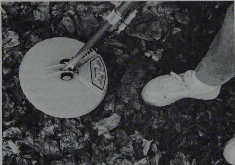
Figure 9-6 Pickup head in a metal detector unit for detecting the location of metallic substances.
