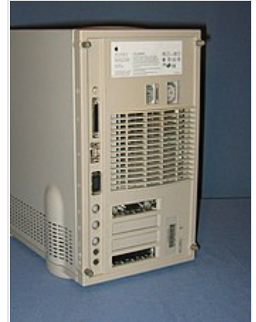
HDI-45 is the third onboard connector from the top along the left rear edge of this Power Macintosh 8100 .
