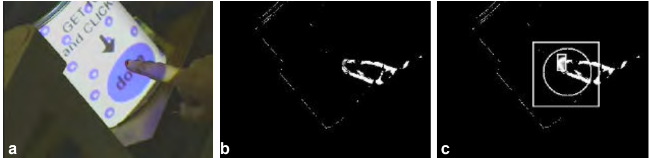
Fig. 4. a) Camera view of an interaction with a bucket; b) image difference data; c) overlay of search region (square), button active area (circle), and the fingertip template shown at the pointing location.
