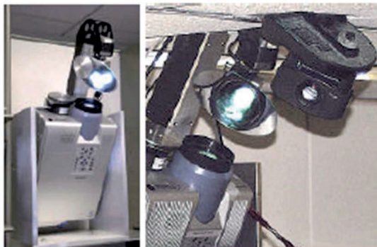
Figure 3. Prototype of the ED-projector: a) ED-projector without the camera mounted; b) a detail of a complete prototype, including the pan/tilt camera.
