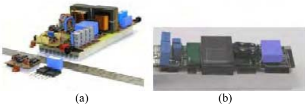
Fig. 22: Comparison among different DC/DC converter designs: (a) 200 kHz AHB, 12\text{W}/\text{in}^3 (b) 1MHz LLC, 76\text{W}/\text{in}^3
