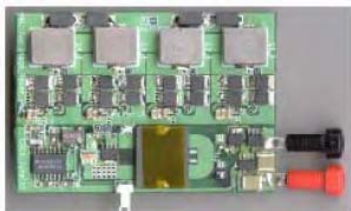
Fig. 32: 130W two-stage power pod prototype for server
