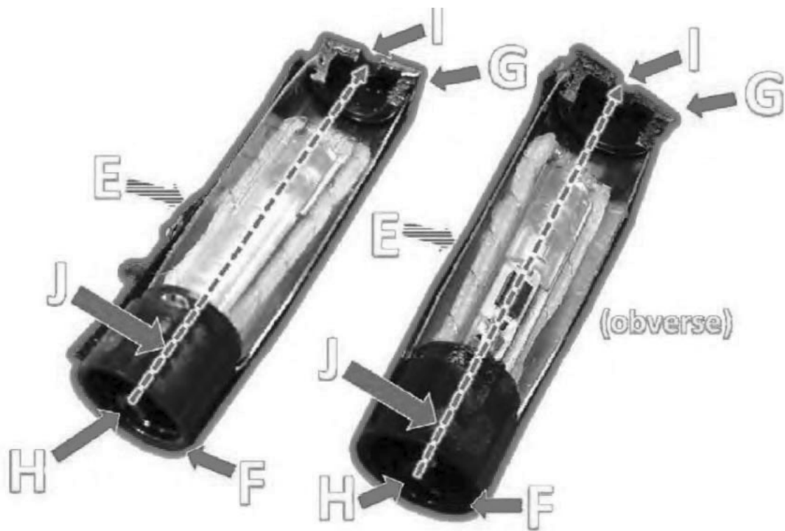
CX-2157 (Vallee Opening Report) ¶ 1869 (Photo of VUSE Solo G1 Cartridge That Includes in Its Housing [E] an Airflow Passageway [J] that Extends Centrally and Axially from a First Aperture [H] to a Second Aperture [I])
