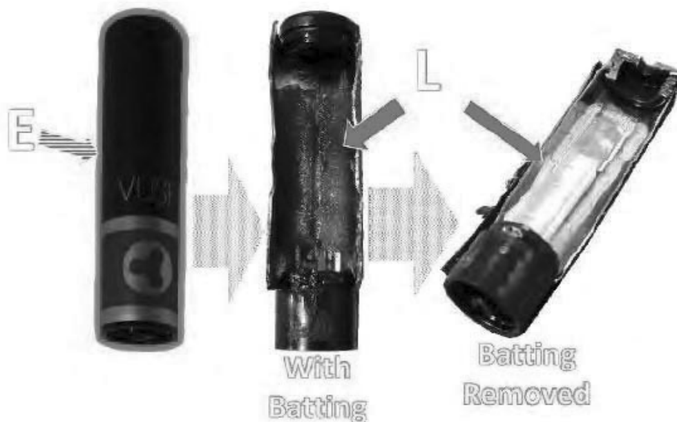
CX-2157 (Vallee Opening Report) ¶ 1880 (Photo of VUSE Solo G1 Cartridge Housing [E] (Left), Interior with Batting [L] (Middle), and Without Batting to Show the Portions of the Wick Outside the Heating Coil [L] (Right))
