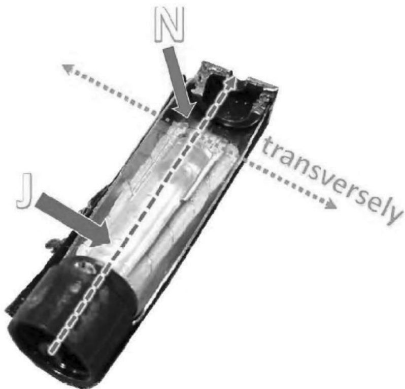
CX-2157 (Vallee Opening Report) ¶ 1886 (Photo of VUSE Solo G1 Cartridge Showing Heating Element [N] that Extends Transversely Across the Airflow Passageway [J])
