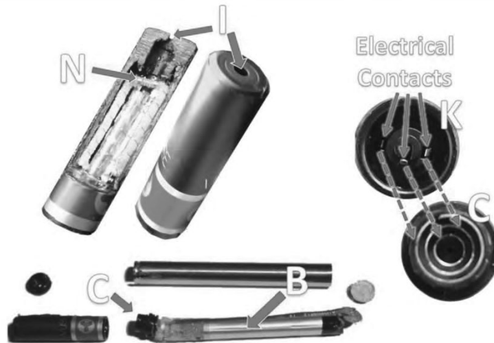
CX-2157 (Vallee Opening Report) ¶ 1906 (Photo of VUSE Solo G2 Cartridge Showing the Cartridge's Electrical Contacts [K] That Couple to the Power Source [C])
