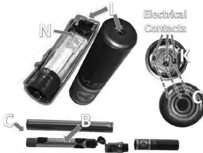
CX-2157 (Vallee Opening Report) ¶ 1906 (Photo of VUSE Solo G1 Cartridge Showing the Cartridge's Electrical Contacts [K] That Couple to the Power Source [C])
