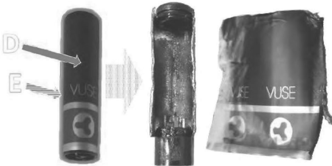
CX-2157 (Vallee Opening Report) ¶ 1864 (Photo of the VUSE Solo G1 Cartridge [D] with Housing [E] (Left), and the VUSE Solo G1 Cartridge [D] with the Housing [E] Removed to Show the Interior (Right))
