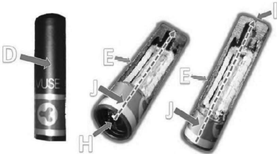
CX-2157 (Vallee Opening Report) ¶ 1869 (Photo of VUSE Solo G1 Cartridge That Includes in Its Housing [E] an Airflow Passageway [J] that Extends Centrally and Axially from a First Aperture [H] to a Second Aperture [I])
