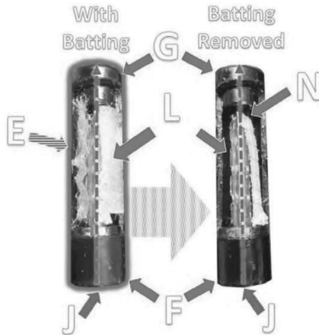
CX-2157 (Vallee Opening Report) ¶ 1892 (Photo of VUSE Solo G1 Cartridge Showing Interior of Housing [E] With a Solution Holding Medium [L] that Surrounds the Airflow Passageway [J] and Heating Element [N] Between the First and Second Ends [F, G])
