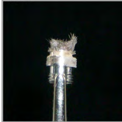
Triple wrapped inverted T configuration
