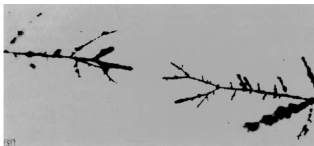
Fig. 8.5 Dendritic growth of “brown smoke” agglomerates (Fig. 8.4) in an electrostatic field [B.48]
