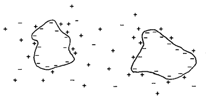
Fig. 8.13 Diagram representation of two particles with electrical double layers in a liquid [B.48]
