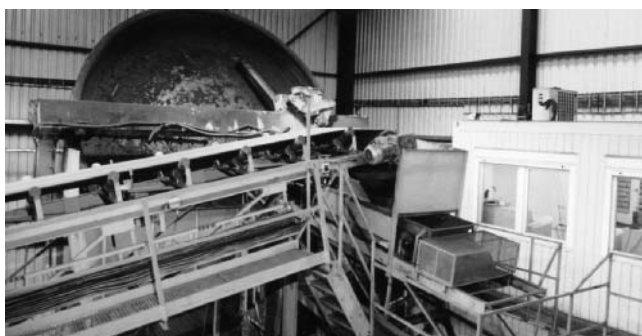
Fig. 8.31 Disc pelletizer for the recycling of waste dusts, slurries, and plant fines (courtesy Heckett MultiServ, Butler, PA, USA)
