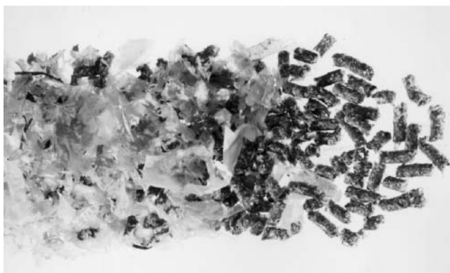
Fig. 8.42 Pelleted secondary fuel, right, from combustible domestic and industrial waste, left (courtesy Amandus Kahl, Reinbek, Germany)
