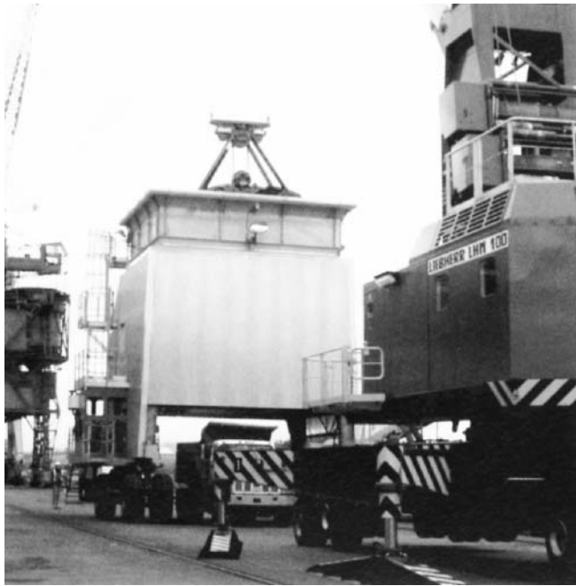
Fig. 8.6 Loading of a truck by heavy duty clam shell grab via dockside mobile loader (DML) to avoid pollution of the environment [8.1.1]
