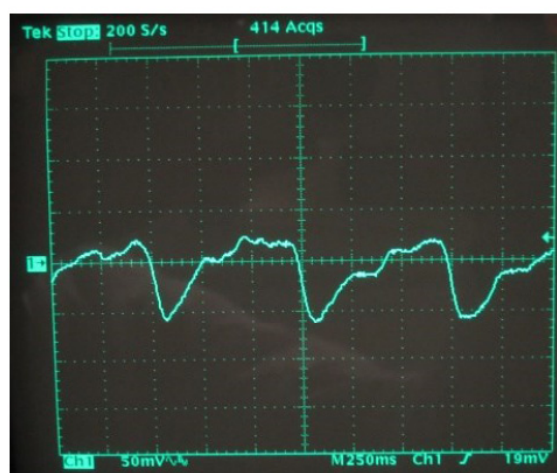
FIGURE 12. The pulse signal obtained by the infrared LED.
