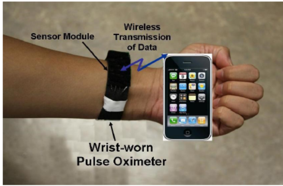
FIGURE 2. Wireless transmission of sensor data from the wrist pulse oximeter.
