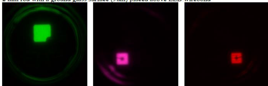
2 mm rod with a ground glass surface (9um) placed above LED wirebond
