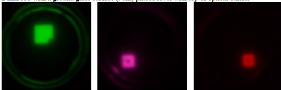
2 mm rod with a ground glass surface (9um) placed level with top of optical barrier
