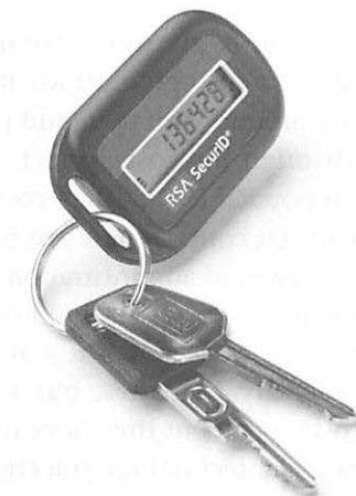
FIGURE 11.5 SecurID token from RSA Security Inc.
