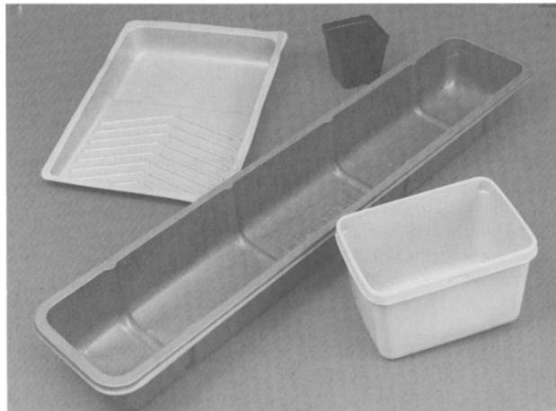
Fig. 13-31. Typical steel-rule die trimmed parts where trim tolerances are not very critical and high-speed production is not a major factor. Usually the forming and trimming are accomplished in one unit. (Courtesy Lyle Industries, Inc.)
