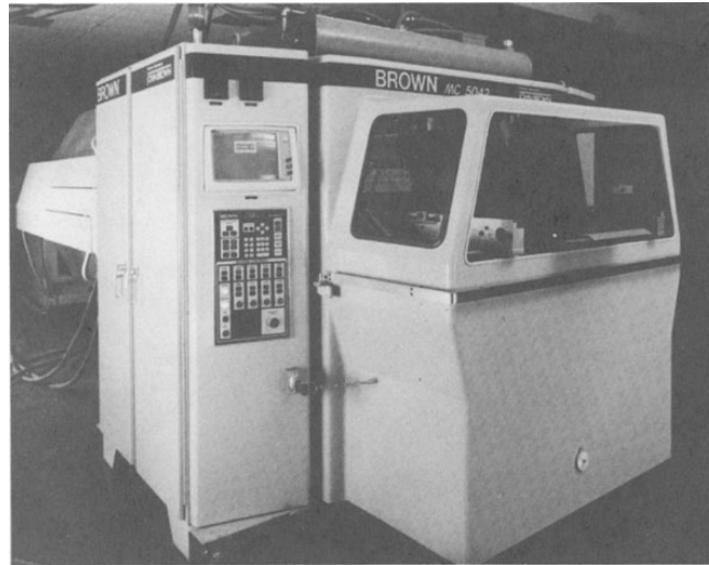
Fig. 13-26. Microprocessor control provides precise and accurate temperature readings automatically, adjusting accordingly to bring sheet to the setpoint temperature. (Courtesy Brown Machine, Div. John Brown)
