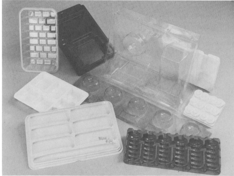
Fig. 13-23. Typical thermoformed blister packaging and box inserts, unusually formed to the shape of the product to be packaged. (Courtesy Lyle Industries, Inc.)
