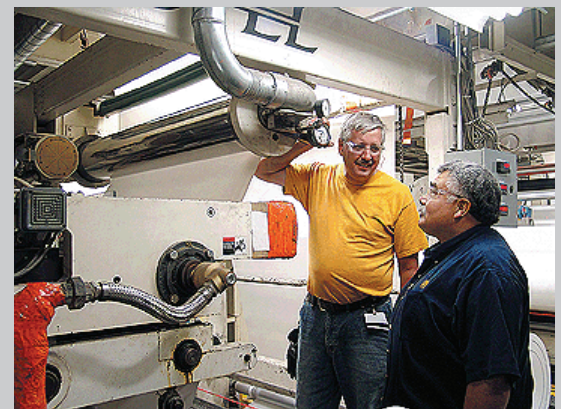
Special projects coordinator Mike Mendolla (right) and operator Rick Gezella are shown with one of the 12 vacuum rolls in use at Green Bay Packaging. This one is positioned immediately after an overhead dryer.
