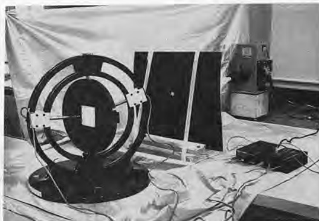
FIGURE 2. Bidirectional solar-optical properties apparatus.
