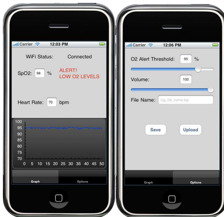
Figure 32: Final user interface GUI implemented on iPod Touch
