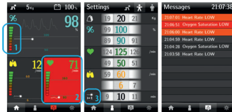
Figure 3 The second Phone Oximeter graphical user interface prototype as used in Phase II of the study. Visual changes made to the interface are highlighted in blue: (1) new signal quality indicator; (2) improved visual alert for alarms; and (3) improved icon for the trend line indicator.
