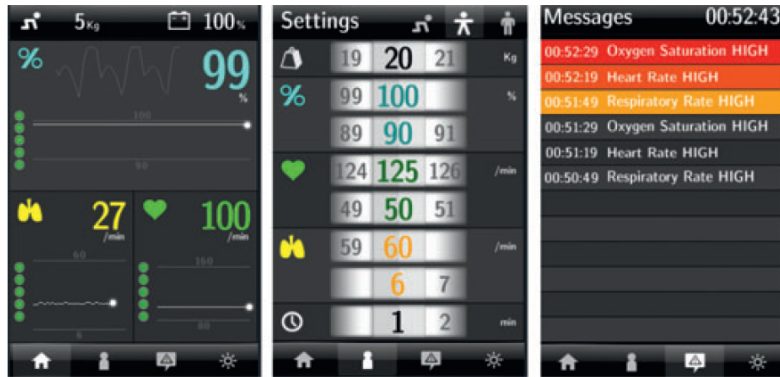
Figure 2 The graphical user interface of the first prototype of the Phone Oximeter is composed of four tabs, which can be selected from the bottom bar (left to right): Home , Settings , Messages and Power-saver (not shown).
