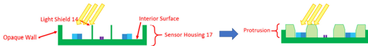
Apple’s fabricated illustration of Mendelson-799 (left, Petition at 13) Apple’s “Mendelson-799-Aizawa” structure (right Petition at 22) (light reflected from measurement site added in yellow)
