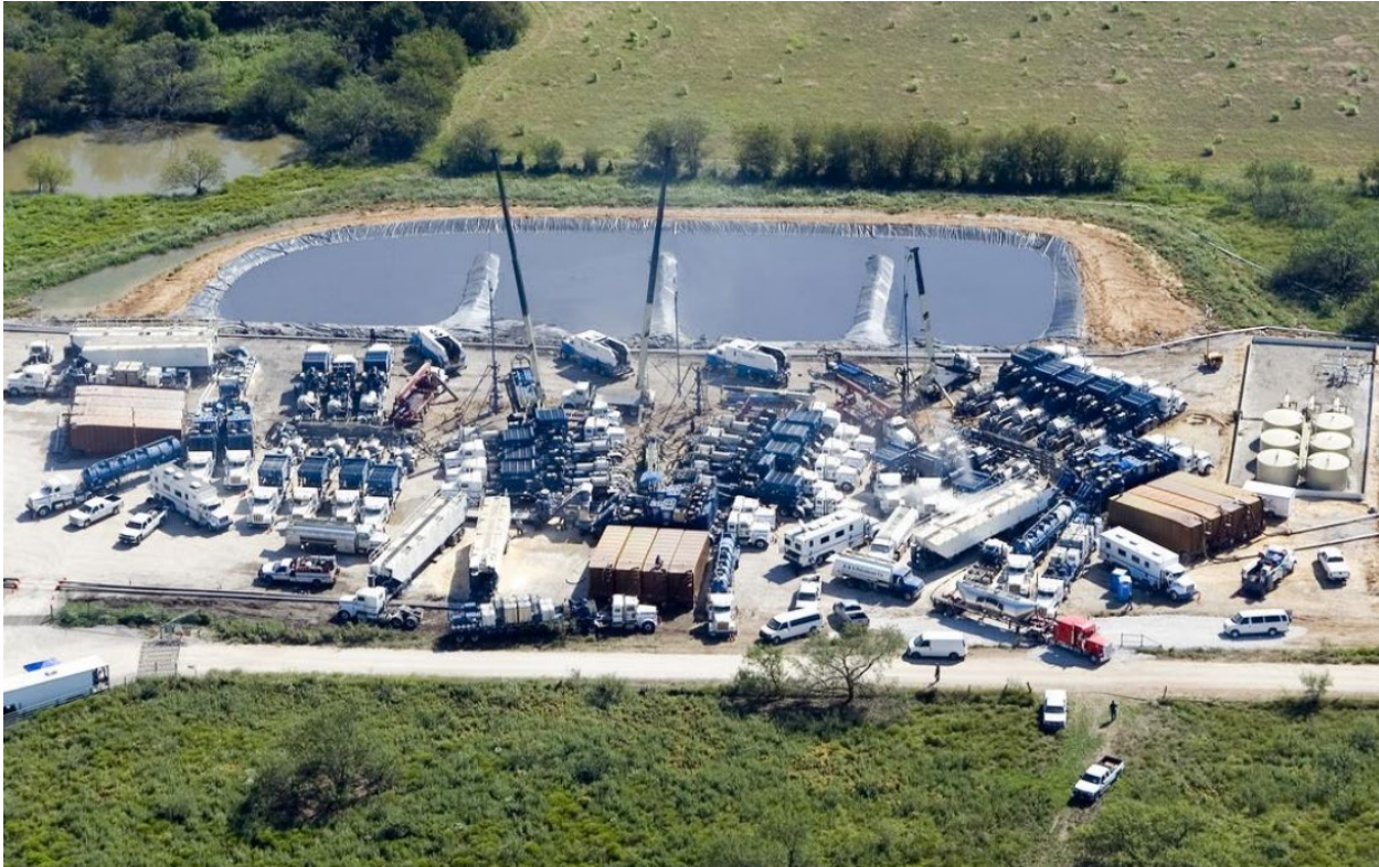
Figure 14 Simultaneous fracture treatments being performed on three Barnett shale gas wells, north of Fort Worth (Source: BJ Services Hydraulic Fracturing hand
