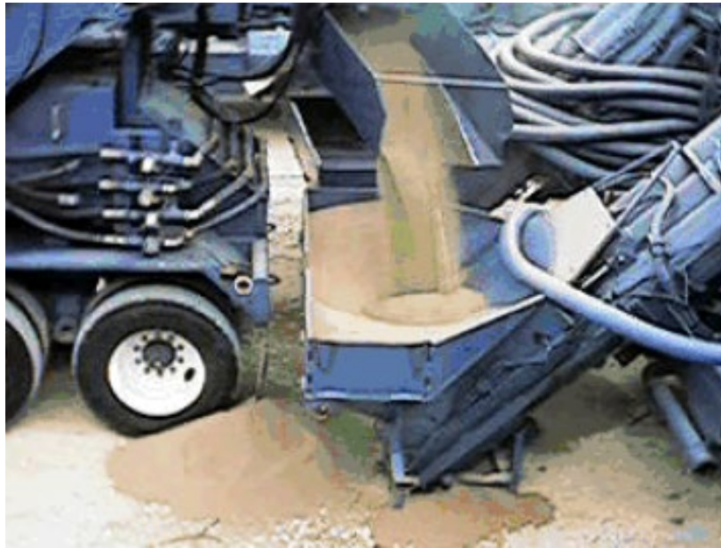
Figure 6 Frac sand being delivered from a Sand King to the blender
