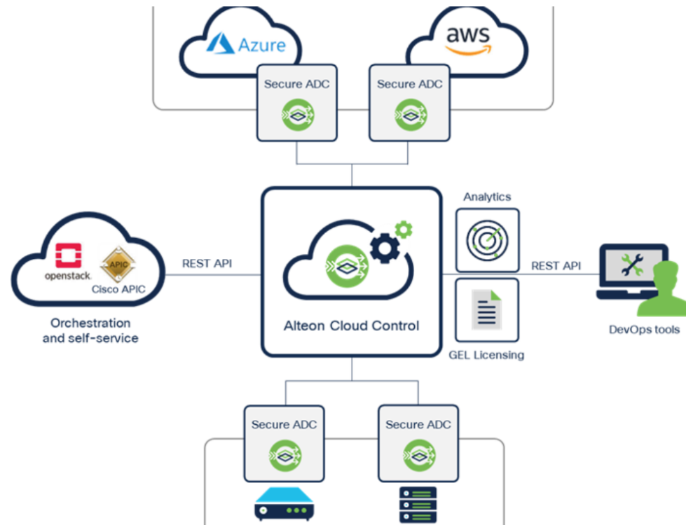
Figure 2. Secure ADC multicloud solution architecture
