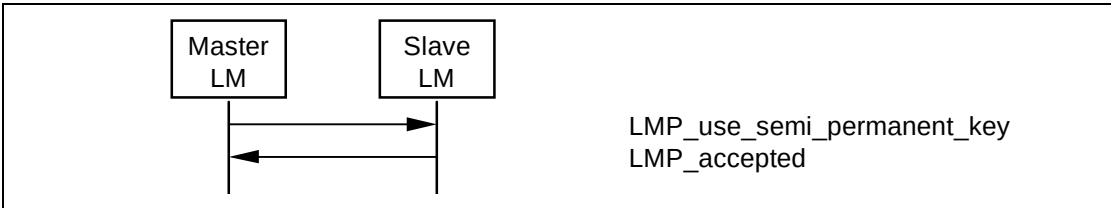
Sequence 11: Link key changed to the semi-permanent link key.
