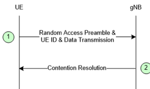
Figure 3: 2-step RACH procedure
