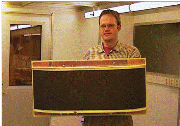
■ FIGURE 5. Picture of an 8-element array antenna at 1.8 GHz. (Antenna property of Telia Research AB, Sweden).
