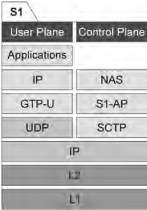
Figure 1.72 Protocol stack S1 control/user plane.
