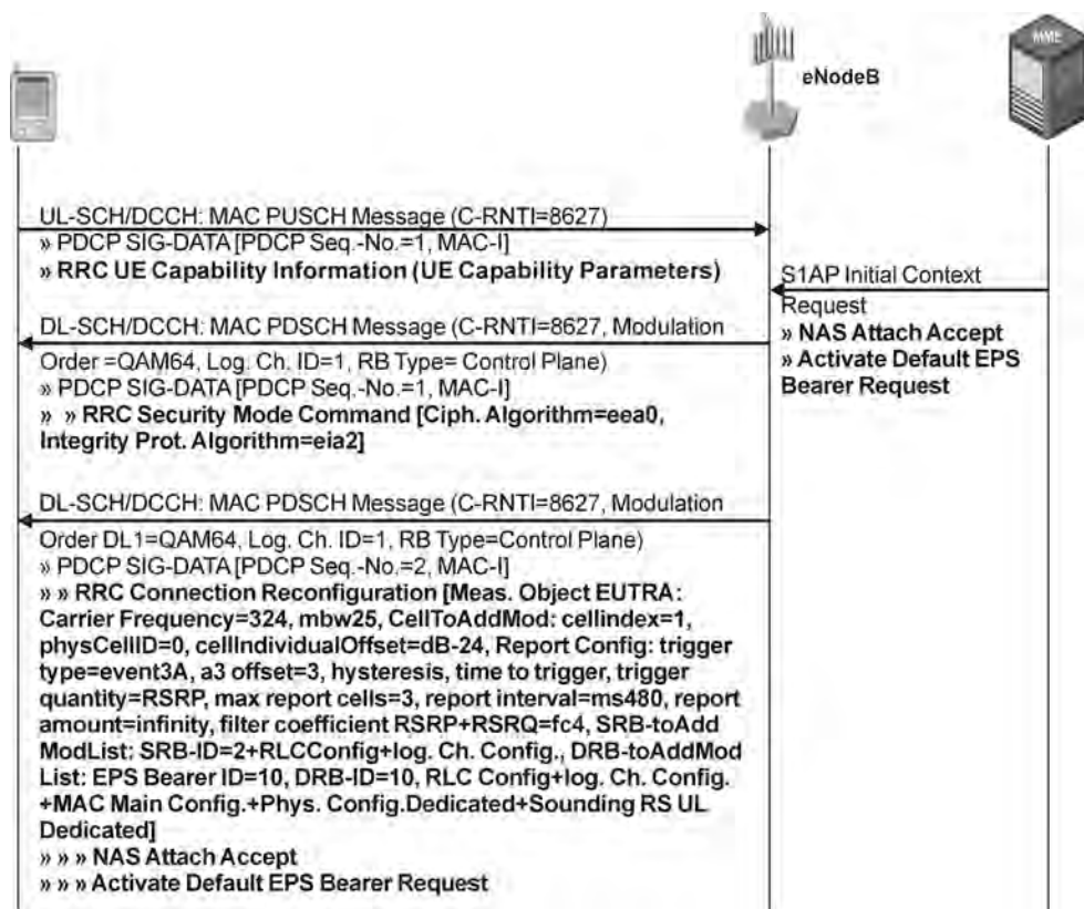
Figure 3.3 RRC connection setup 2/3. (Tektronix Communications).
