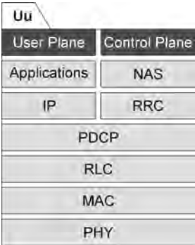
Figure 1.71 Protocol stack LTE Uu interface.
