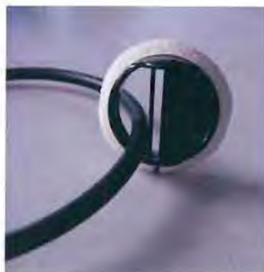
Figure 4.5.1 Valve obstructed by o-ring cord
