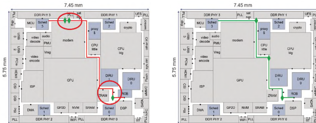
Figure 9.5. Pipeline stages are required in a path to span a particular distance given the clock period and transport delay (Arteris IP 2020)
