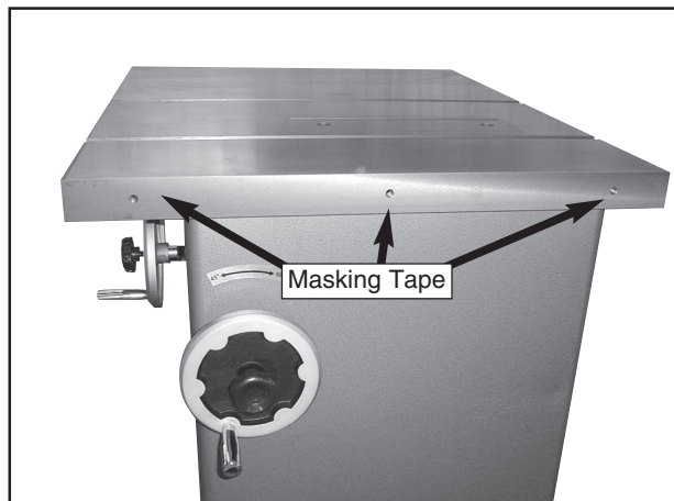
Figure 7. Using tape to shim for wing alignment.
