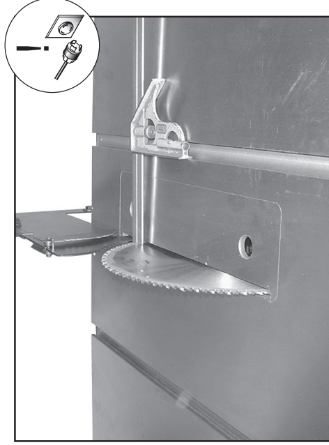
Figure 21. Measuring for parallelism.
