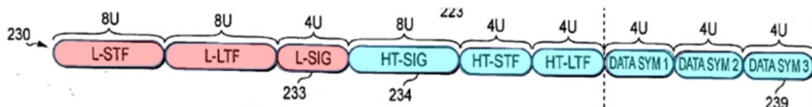
Ex. 1011, Fig. 2 (excerpted and color-coding added) Trainin's Mixed Mode Frame Format
