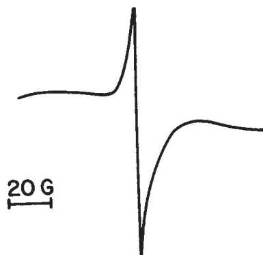
Fig. 2. ESR signal of a plasma polymer of tetramethyldisiloxane (without glass signal).
