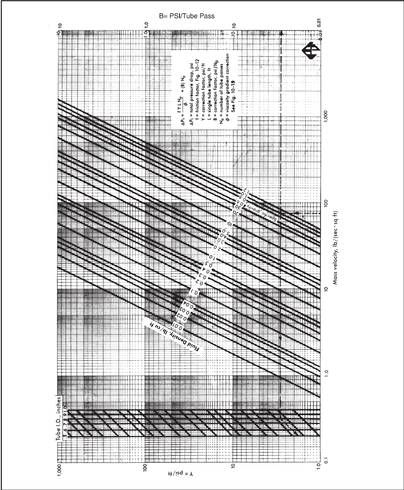
FIG. 10-14 Pressure Drop for Fluids Flowing Inside Tubes
