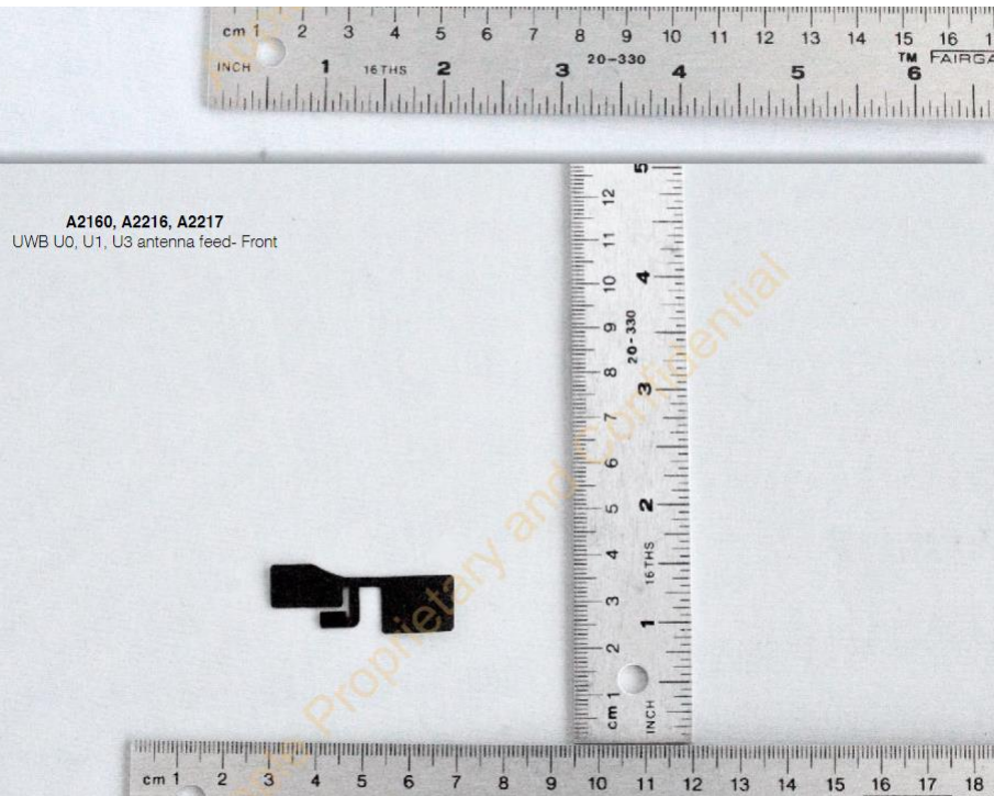
iPhone 11 UWB (ultra-wideband) antenna feed showing 2 antennas ( https://fccid.io/BCG-E3305A/Internal-Photos/Internal-Photos-4423150 )
