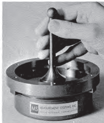
Fig. 5.5 Rigid joystick (courtesy Measurement Systems, Inc.).
