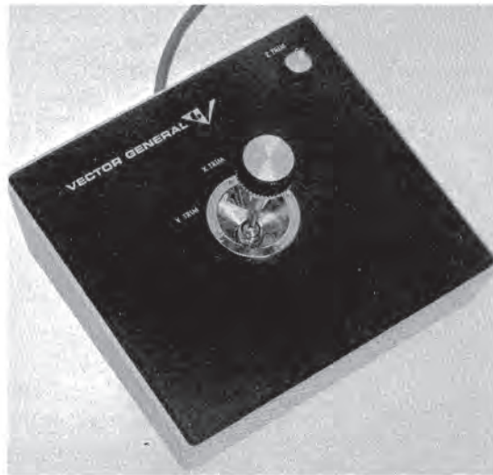
Fig. 5.4 Joystick with rotating shaft to provide third axis (courtesy Vector General).
