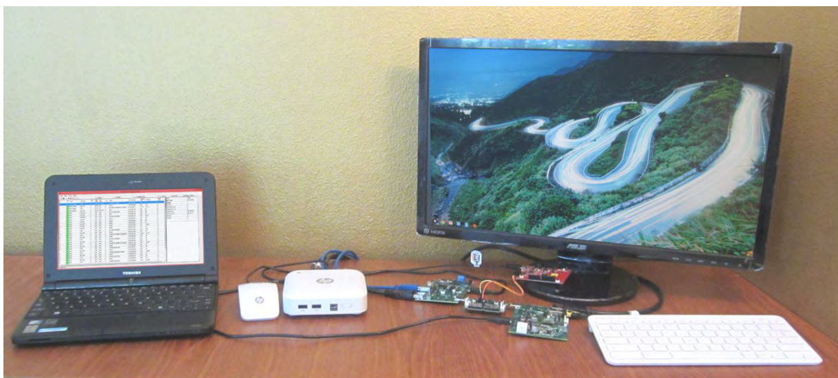
Figure 16. Chromebox PC and Three CY4501 CCG1 Development Kit Boards with Debug Laptop
