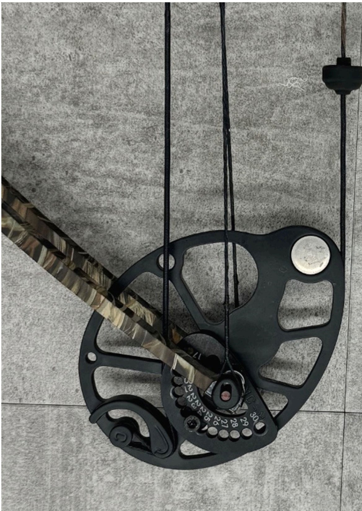
Photo 5: Menace '817 bow lower cam in brace condition.
