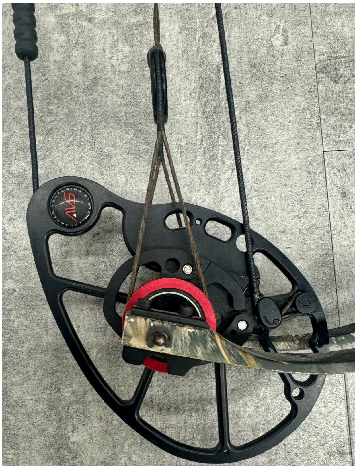
Photo 4: Monster '775 bow lower cam in brace condition.
