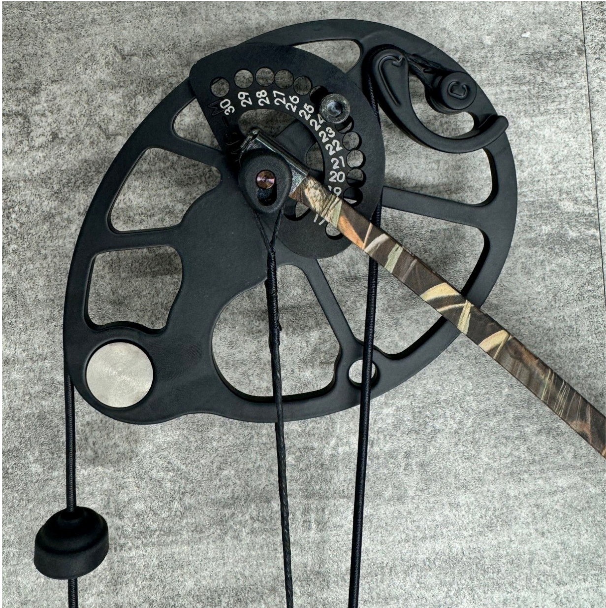
Photo 4: Menace '455 bow upper cam in brace condition.
