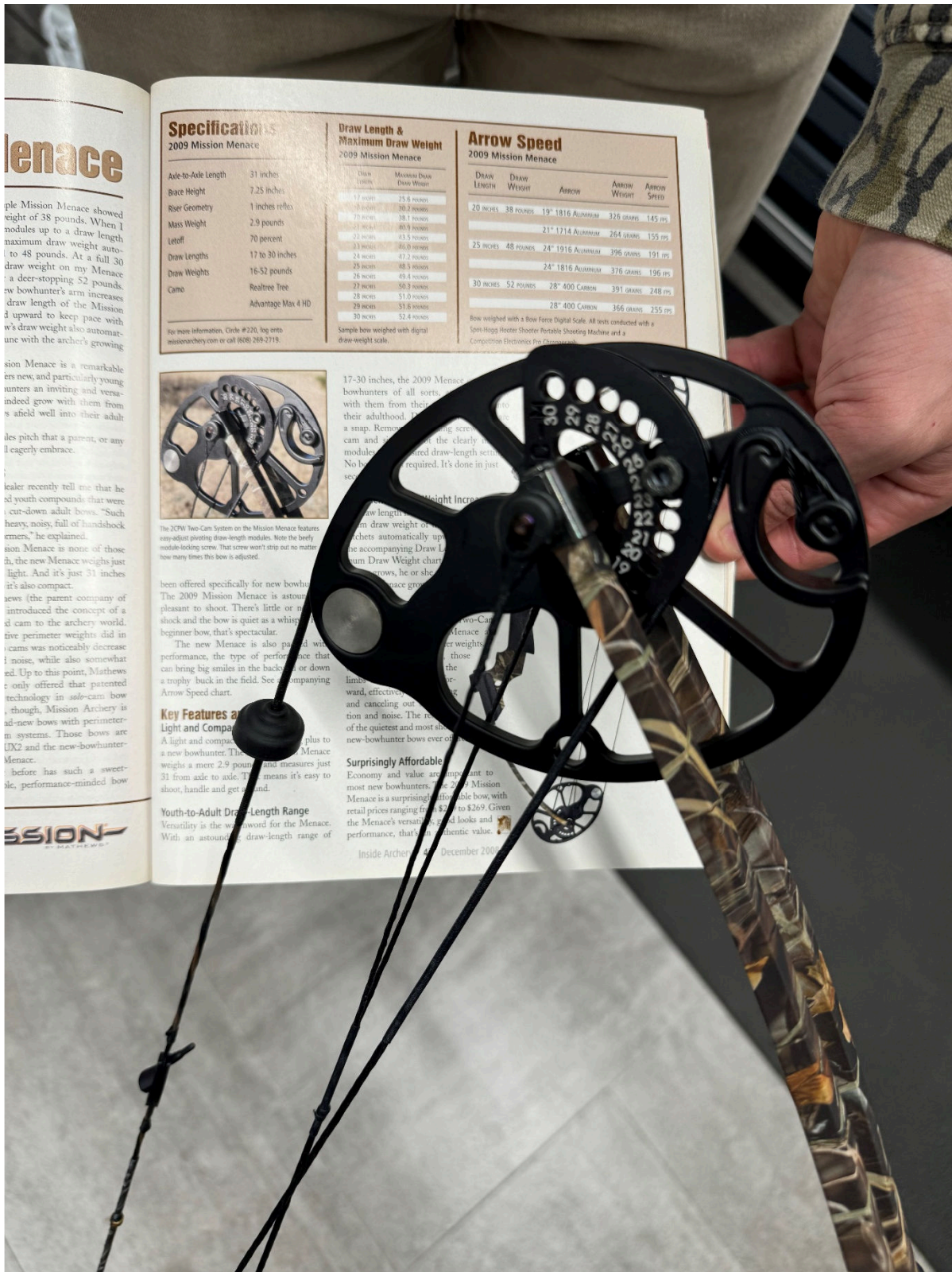
Photo 7: Menace '455 bow lower cam in brace condition next to a cam photograph in 2009 Mission Menace article of the Inside Archery December 2008 issue.
