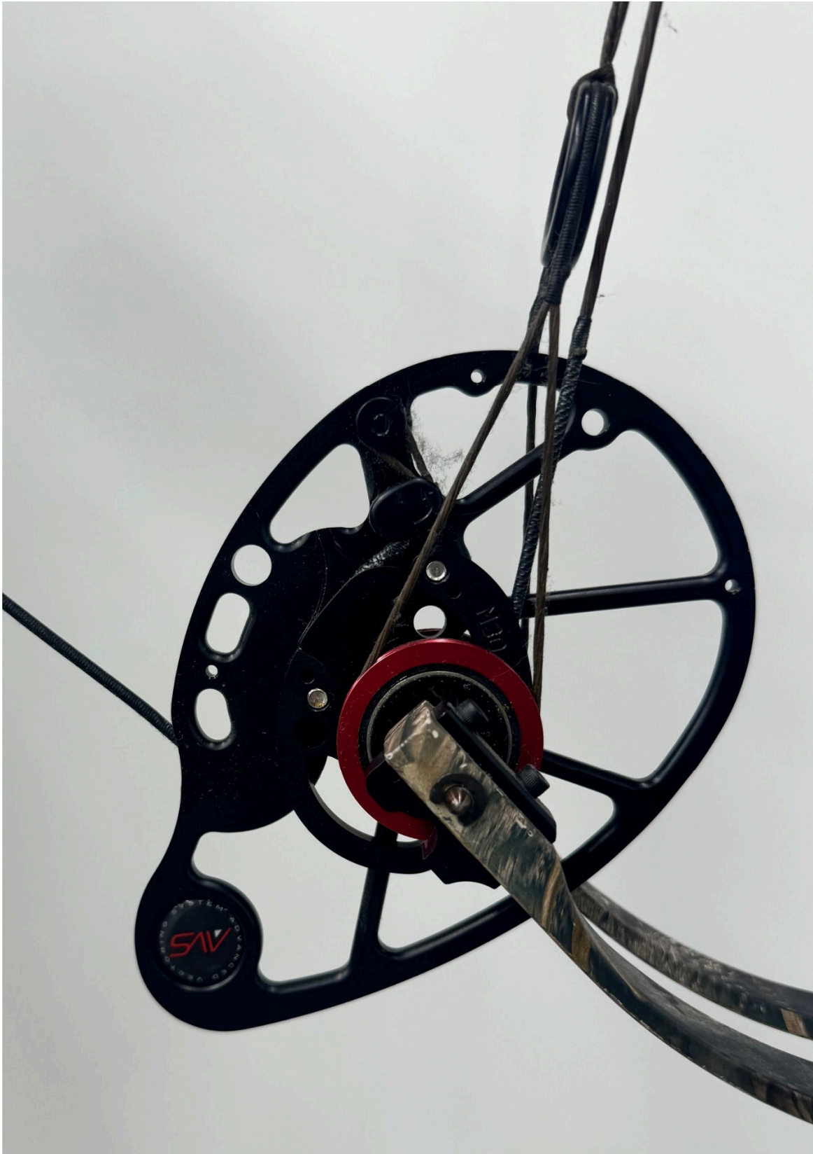
Photo 7: Monster '775 bow lower cam in drawn condition.
