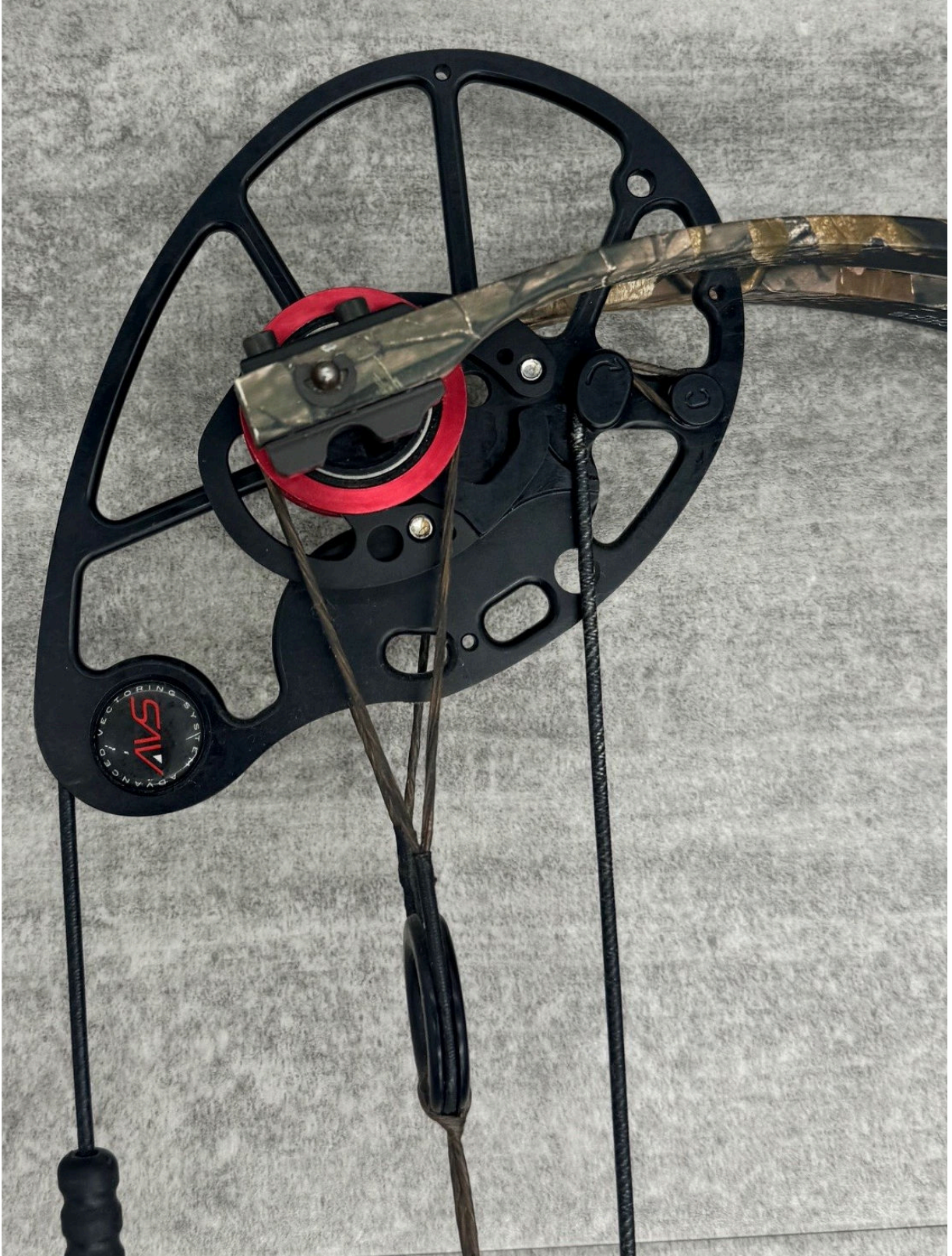
Photo 3: Monster '775 bow upper cam in brace condition.
