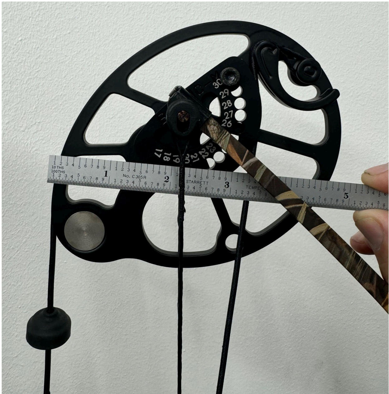
Photo 3: Menace '817 bow upper cam in brace condition.
